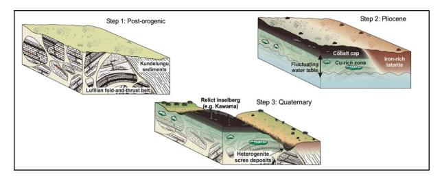
Figure 7: Sketch diagrams illustrating the three major steps in the formation of secondary oxidized Co ores in Katanga (vertical scales are exaggerated). Source: Decrée et al. 2010a
