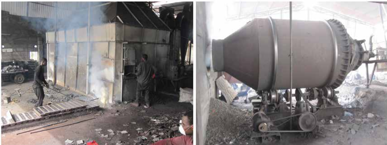
Figure 4-6: Two major types of secondary lead furnaces: Blast furnace (left), rotary furnace (right)
