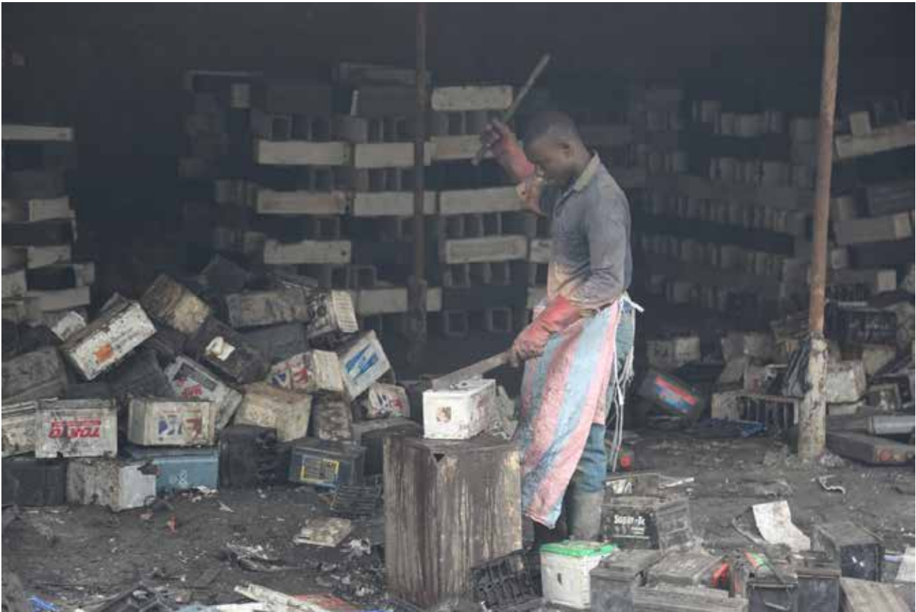
Figure 4-3: Opening of drained lead-acid batteries to extract lead-scrap
